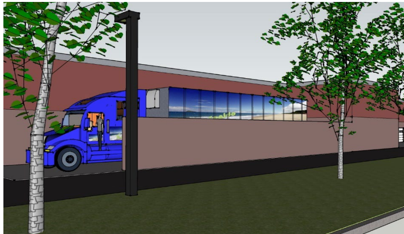
Figure 15.14.050-8: Service area screened by an 8' masonry wall.
