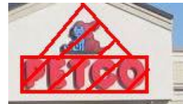
Figure 15.14.120-10: Wall sign display area. The hatched area represents the sign display area.
