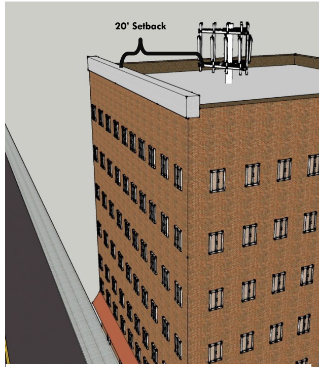
Figure 15.14.130-3 Rooftop towers and antennas shall be camouflaged if located within 20' of the roof's edge.
