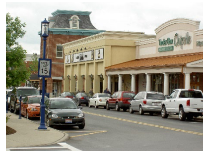
Figure 15.14.060-10: Separating pedestrians from traffic and the elements through the use of arcades
